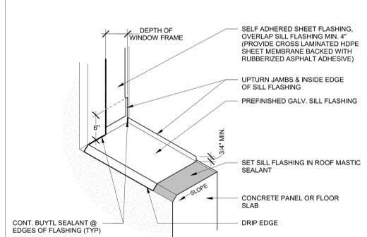
**TYP FLASHING @ WALL OPENINGS**
